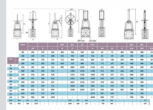
Dimensions are for guidance only – detailed dimensions drawings available on request. All dimensions are in millimeters, unless stated.
